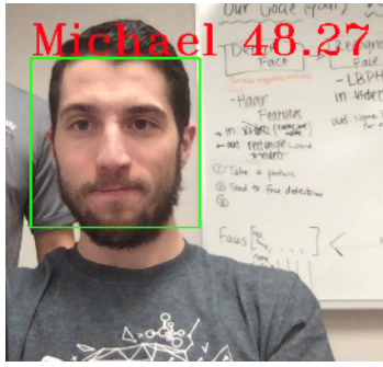
Fig. 3. After face detection, facial recognition is performed using LBPH classification, and an error score is computed.
