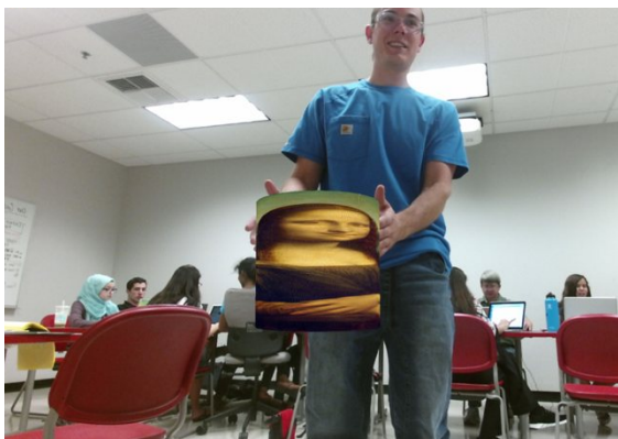
Fig. 3. Live video feed being overlaid with a virtual cylinder wrapped in Leonardo Da Vinci's Mona Lisa
