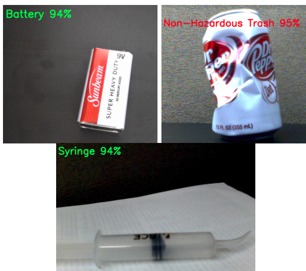
Fig. 6. The accuracy of the CNN classifying the battery, non-hazardous trash, and syringe
